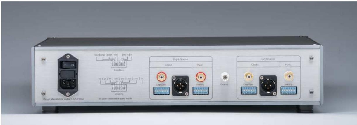
The XP-17 does not differentiate between moving magnet (MM) or moving coil (MC) phono-cartridges you will simply be setting gain as is appropriate for your specific cartridge. In all instances the switch-tab for any selection will need to be up for "on" and down for "off".
