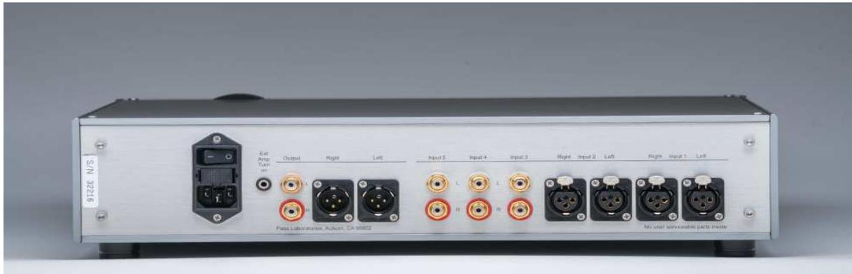
We have provided a standard IEC AC power cord that fits into the IEC 320 line receptacle at the rear of the preamplifier chassis. The preamplifier is equipped for operation with an earth ground provided by the users AC outlet. Do not defeat this ground.
