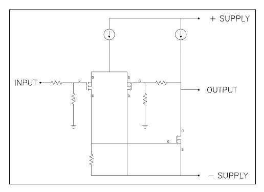
Mosfets provide the widest bandwidth of solid state power devices, however they were not chosen for this reason. The design of the Aleph 5 does not seek to maximize the amplifier bandwidth as such. The capacitances of the Mosfets provide a natural rolloff in conjunction
