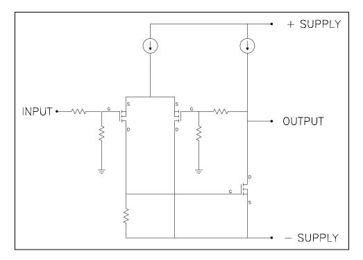
Mosfets provide the widest bandwidth of solid state power devices, however they were not chosen for this reason. The design of the Aleph 3 does not seek to maximize the amplifier bandwidth as such. The capacitances of the Mosfets provide a natural rolloff in conjunction with the resistive impedances found in the circuit, and the simplicity of the circuit allows for what is largely a single pole rolloff characteristic.
