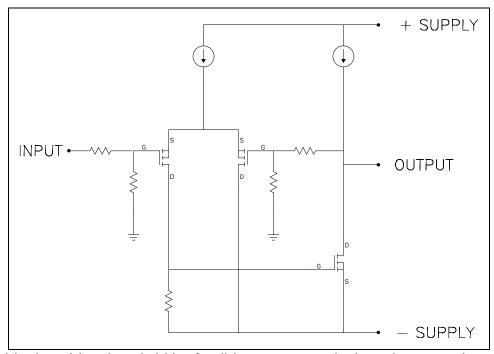
Mosfets provide the widest bandwidth of solid state power devices, however they were not chosen for this reason. The design of the Aleph 30 does not seek to maximize the amplifier bandwidth as such. The capacitances of the Mosfets provide a natural rolloff in conjunction with the resistive impedances found in the circuit, and the simplicity of the circuit allows for what is largely a single pole rolloff characteristic.
