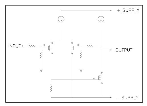
Mosfets provide the widest bandwidth of solid state power devices, however they were not chosen for this reason. The design of the Aleph 1.2 does not seek to maximize the amplifier bandwidth as such. The capacitances of the Mosfets provide a natural rolloff in conjunction with the resistive impedances found in the circuit, and the simplicity of the circuit allows for what is largely a single pole rolloff characteristic.
